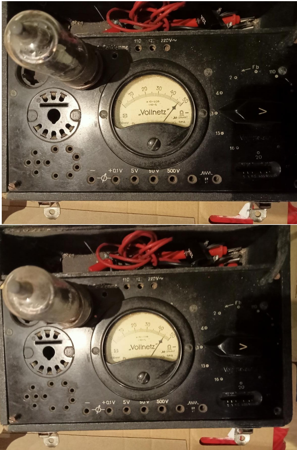
6K8GT (through adapter Octal to CT8). The lower valve has some weakness around the base. The 6K*GT was first introduced in 1938 https://www.r-type.org/exhib/aaq0104.htm
